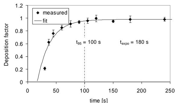
Figure 1. Time course of aerosol deposition onto cells in the ALICE-CLOUD (Aeroneb Pro nebulizer). The asymptotic deposition factor of 0.836 implies that 83.6% of the invested liquid reaches the bottom of the chamber, where the cells are positioned.
