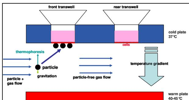
Figure 1. Concept of the Cyto-TP, a combination of a thermal precipitator and the air-liquid interface technique
