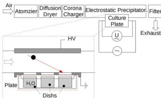
Figure 1. Setup for dosimetry measurements with sodium chloride aerosol.
