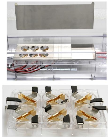
Figure 2. Top: Side view of precipitator with lid open. Bottom: 6-well culture plate equipped with conductive electrodes for on-line conductivity measurements.
