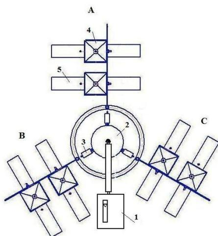
Figure 1. Conceptual top view AECI ( A, B, C – AECI dynamic channels, 1- systemic aerosol generator, 2- shaper of the primary aerosol, 3- mixer of the aerodispersed flows, 4- dynamic subchannels, 5- animal restraining devices.
