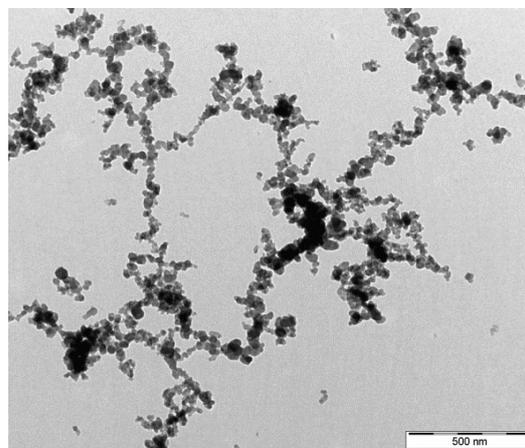
Figure 1. TEM images of diesel fuel inside the VITROCELL<sup>®</sup> Module of HICE exposure system while an exposure experiment at the ship diesel in Rostock
