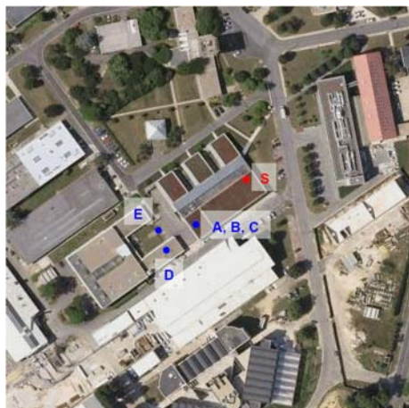
Figure 1. Sampling sites selected from predictions of the distribution of aerosols generated from the source (S). A, B, C were located at 50 m from the emission, D at 70 m on another roof and E at 70 m at the ground.
