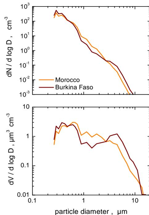
Figure 1. Size distribution of dust from Morocco and Burkina, re-suspended in the aerosol chamber of AIDA and measured downstream a cyclone.
