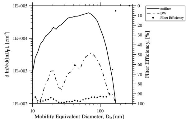
Fig. 2. Example for a typical number size distribution of laser printer emissions; unfiltered (nofilter) and filtered using the Dexewet filter system (DW).
